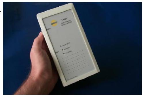
Control unit for antenna tuning of base and complementary antennas for the first setup of OBID i-scan long-range applications or the adaption on changed surrounding conditions.
